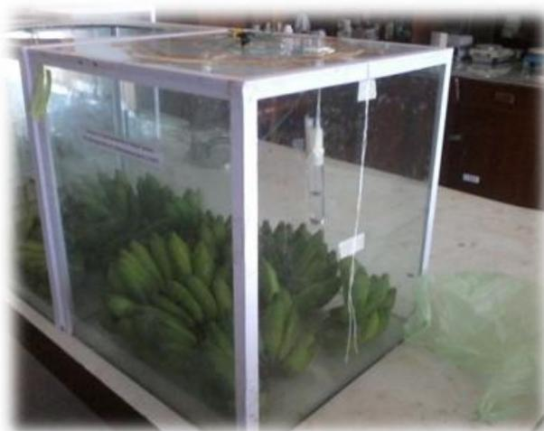
**Figure 1. Glass chamber used for 1-MCP treatment**
