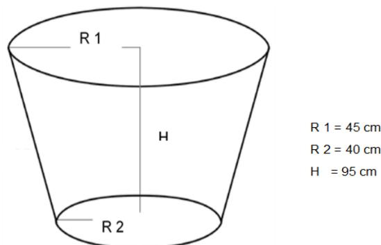
Figure 3. Dimensions of broodstock tanks
