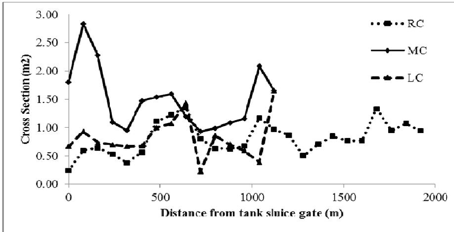
**Fig. 2. Variability of canal cross sectional area with distance**
