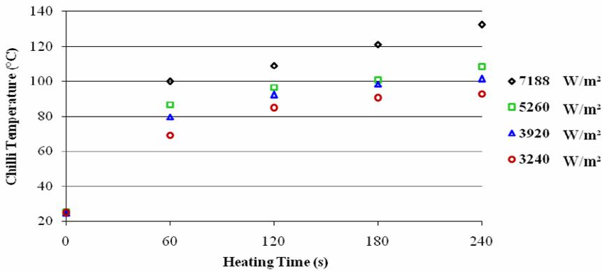
**Fig. 3. Relationship between chilli temperature and heating time under different radiation intensities.**
