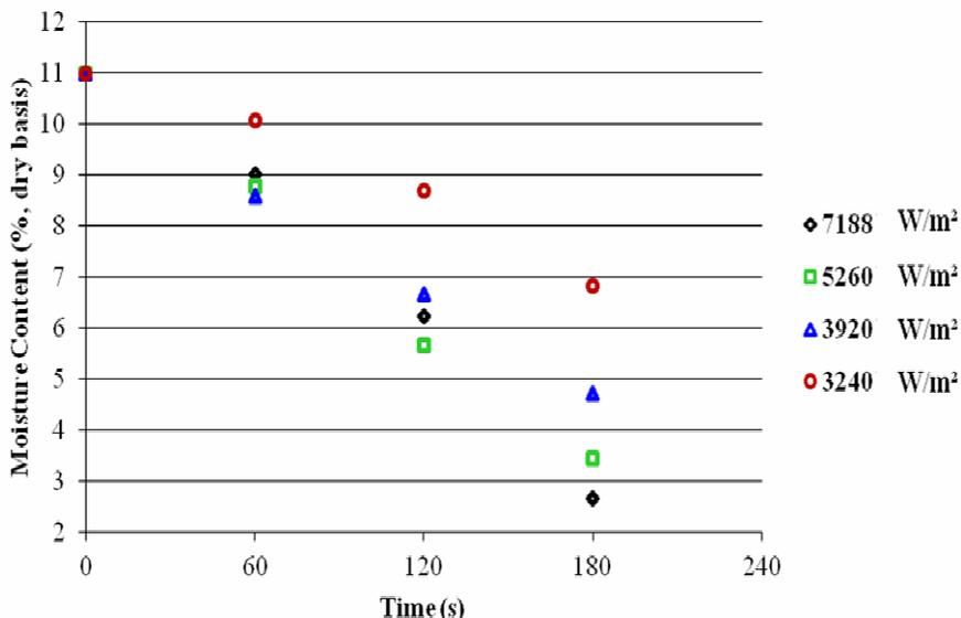
**Fig. 2. Relationship between average chilli moisture content and FIR heating time under different radiation intensities.**
