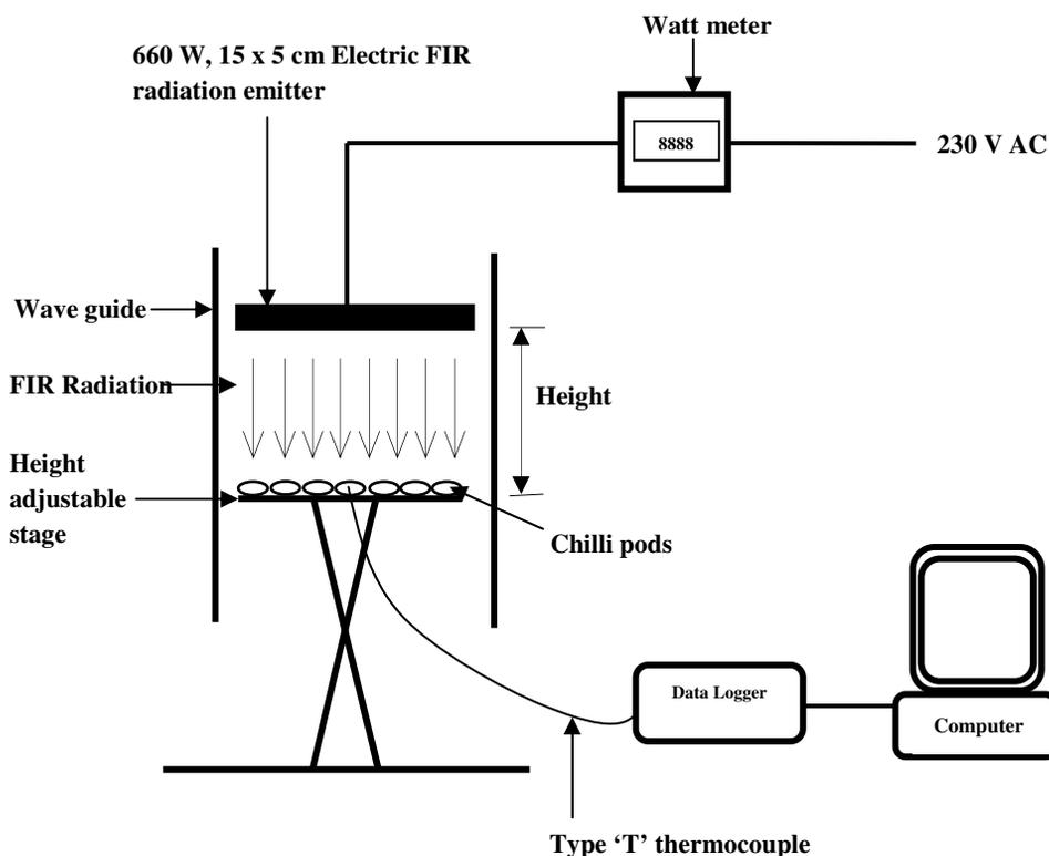
**Fig. 1. Schematic diagram of the FIR chilli roasting setup.**
